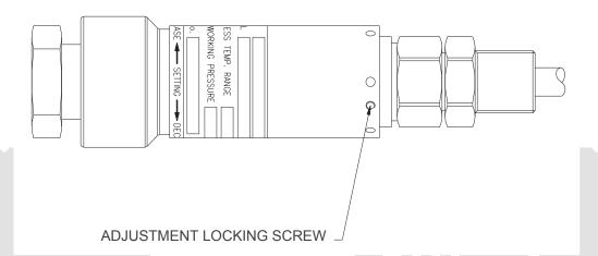
The design features a simple form of adjustment. This enables users to order switches set at a predetermined point or stock a mid range setting and adjust switches to suit the particular application. Rotating the outer tube compresses the discsprings. Rotation clockwise will increase the set point and conversely rotating anti-clockwise will decrease the set point.
